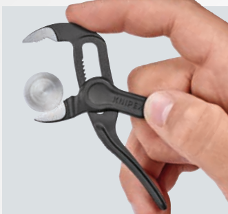
Amazing flexibility: The self-locking effect of the KNIPEX Cobra® XS enables it to grip round materials up to Ø 28 mm extremely reliably – and, due to its very slim head, it can also hold small components in place.
