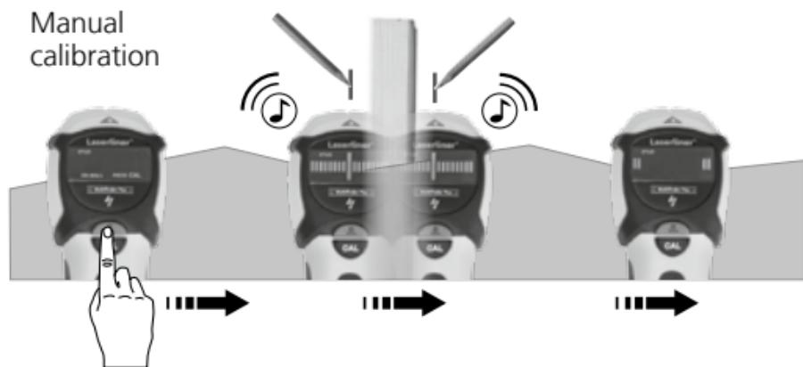
Tip 1: The position between the two markings is the mid-point of the stud.
