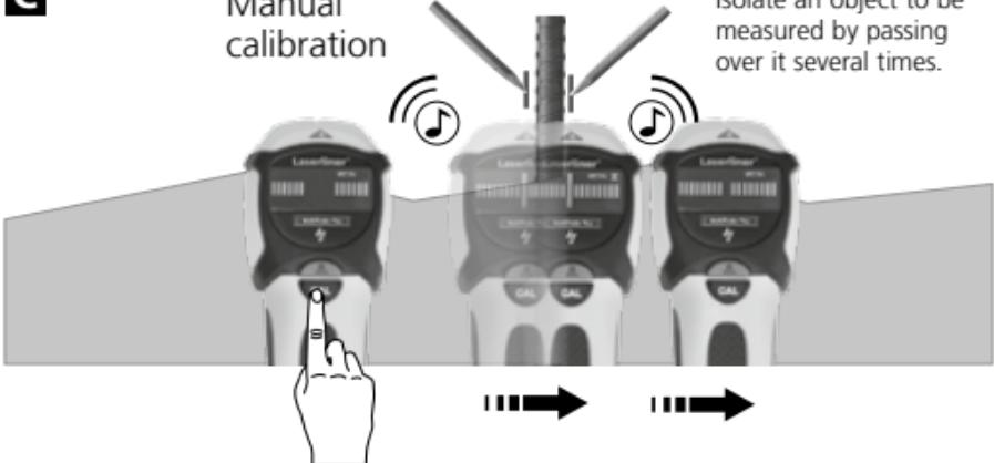
Tip 1: The position between the two markings is the mid-point of the metal object. Through the high measuring sensitivity, thick metal objects appear broader than they are in real life. Therefore move the device over the newly found object as shown in Image B. The device is calibrated automatically during this process. Manual calibration should be performed near the place found last as shown in Image C. Repeat this step as needed.
