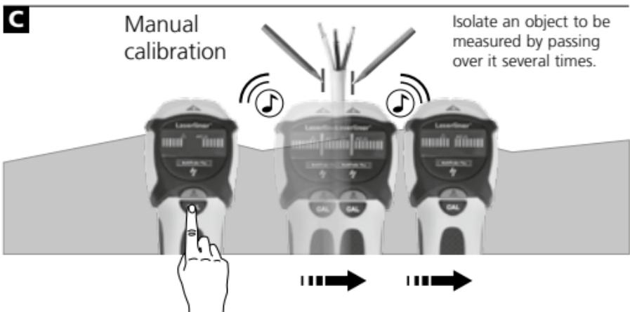
Tip 1: Manual calibration should be performed near the place found last as shown in Image B/C. Repeat this step as needed.
